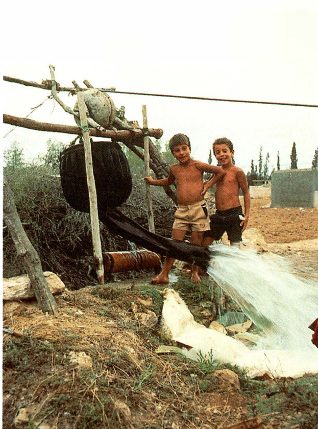
Plate II,12: With this simple system approximately 110 litres of irrigation water are lifted from a depth of 45 m, which takes about three minutes. In a five-hour working day this animal draws some 11,000 water for the irrigation of vegetable plots.
